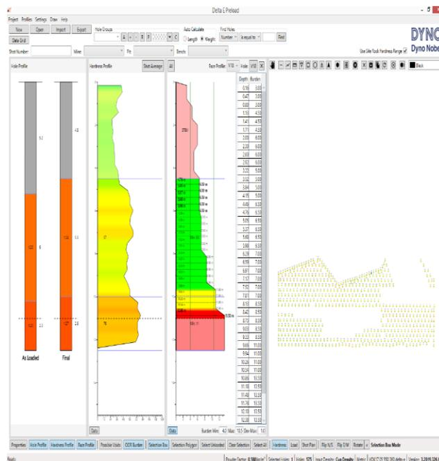
The system can load up to four distinct segments in each blasthole in a single pass. Measurement While Drilling (MWD) data is captured and set to a specific energy requirement using  $\Delta E^2$  software, to optimise design with the required energy placement in each blasthole. The aim is ultimately to improve the overall blasting outcomes.
